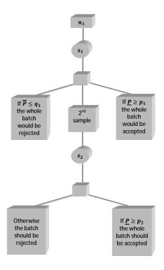
Figure 2.2: Sampling Procedure
