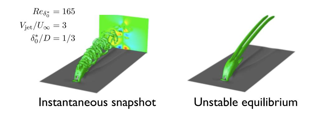
Compute global modes, compare frequencies with observed frequencies in shear layer and near-wall fluctuations
