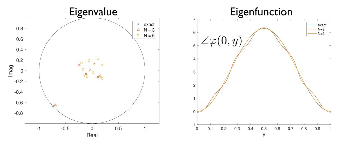
Apply DMD to separated flow past a flat plate
