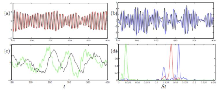
FIGURE 19. The temporal behavior of POD modes are show in terms of the POD coefficients. (a) POD coefficients of the first pair, (b) second pair and (c) third pair of modes. The power spectrum of the signals in (a,b,c) is shown with the same color.
