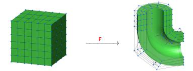
The geometry Ω and its NURBS parametrization F is "given" by CAD general geometry: unstructured collection of "patches".
