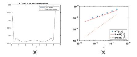
Panel (a) shows the plot of the absolute value of the far field for both models for  $\delta = 0.05$ . Panel (b) shows the far field  $L^2$  relative error  $e^{\infty}(\delta, d)$ , for different values of  $\delta$  and d = (1, 0). The approximated rate of convergence is  $O(\delta^1)$ .
