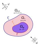
In  $\Omega_{ext}$ ,  $\Omega_+$  and  $\Omega_-$  we have the same equations and on  $\Gamma_1$  and  $\Gamma \setminus \Gamma_0$  the same transmission conditions as for the healthy material.
