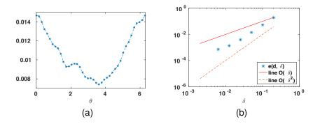
Panel (a) shows the  $H^1$  relative error of total fields resulting from different incident direction. The maximum error is obtained for d = (1, 0). Panel (b) the  $H^1$  relative error for different values of  $\delta$  and d = (1, 0). The approximated rate of convergence is  $O(\delta^{1.7})$ .
